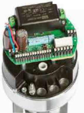
View without cover showing the baelz 7022 circuit board (230 V version)
